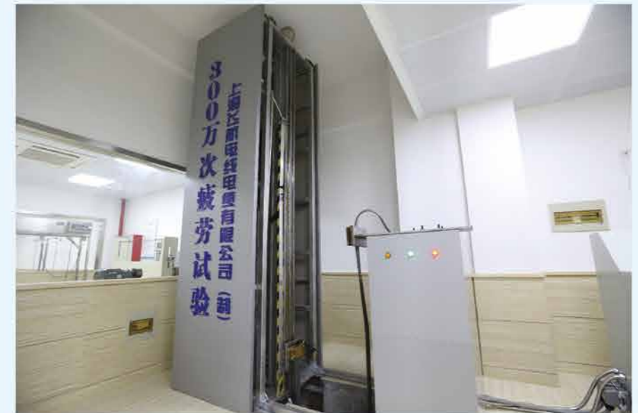
电梯电缆疲劳模拟试验 Fatigue Simulation Test of Elevator Cable
