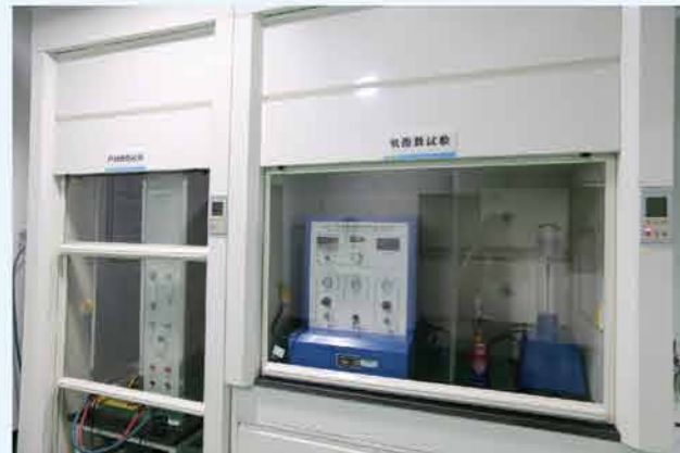
氧指数和单根阻燃试验 Oxygen Index and Single Flame Retardant Test
