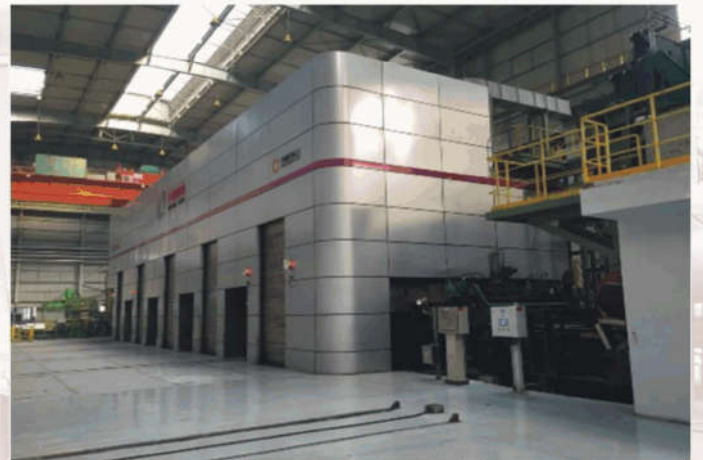
为包钢制造的2030mm酸洗-冷连轧机组 (轧机段) 2030mm PL-TCM for Baotou Steel (rolling mill section)
