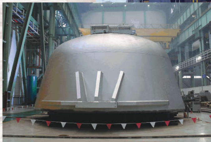
300吨转炉炉壳 furnace shell of 300T Converter
