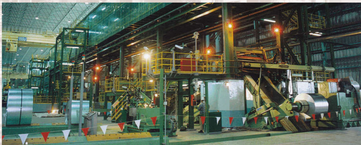
为宝钢制造的1550mm连续电镀锌机组-开卷区 Pay-off reel section, 1550mm Continuous galvanizing line for Baosteel
