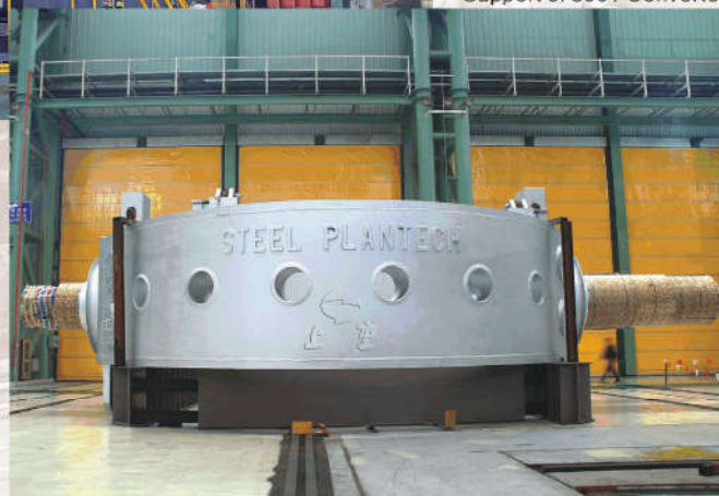
300吨转炉拖圈 Support of 300T Converter
