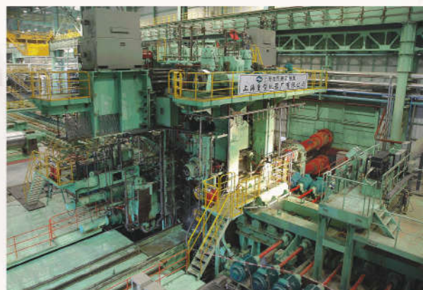
粗轧机 (含立辊轧机) Roughing mill (incl. edger roll)
