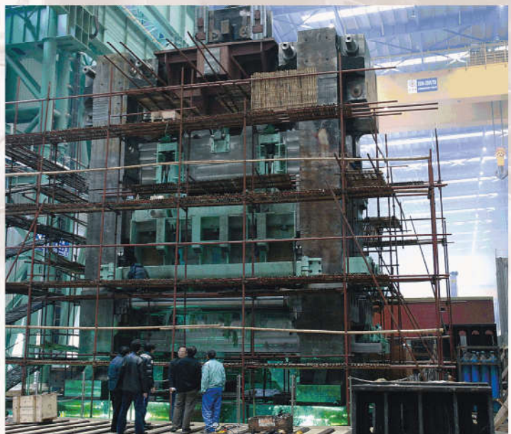
为沙钢制造的5000mm宽厚板轧机(含立辊轧机)(二期) 在上重公司进行出厂装配 5000mm heavy plate mill for Shagang Group (incl. edger, 2nd stage project), assembly in SHMP for delivery
