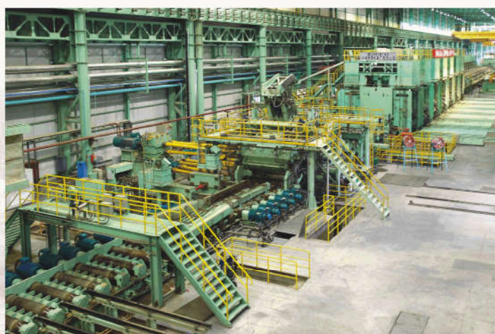
为鞍钢朝阳自主设计制造的1700mmASP热连轧机组 1700mm ASP self-designed hot tandem rolling line for Chaoyang, Ansteel
