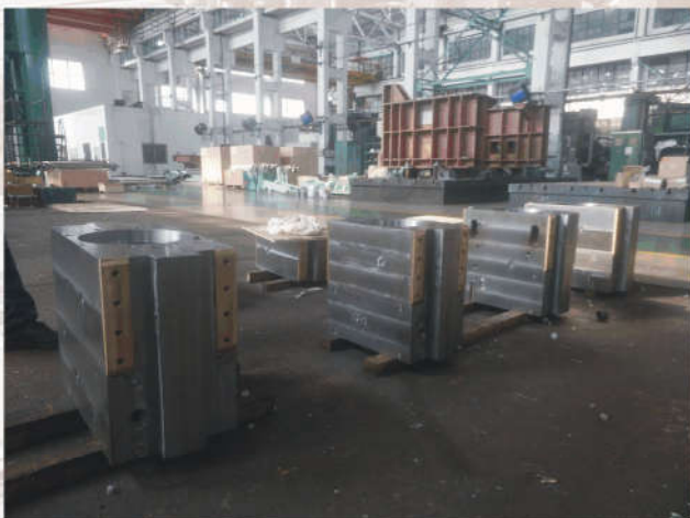
为青海平安铝业制造的铝轧机工作辊轴承座 Work roll chocks for Aluminum plate mill of Pingan Industry Qinhai
