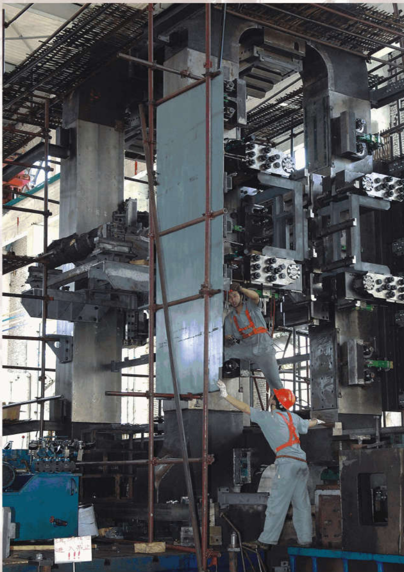
与日本SPCO公司联合设计并制造的台湾烨辉1700mm六辊可逆冷轧机组在上重工厂出厂装配 1700mm 6-high reversing cold rolling mill joint- designed with SPCO and manufactured for Yehui Taiwan assembly in SHMP for delivery
