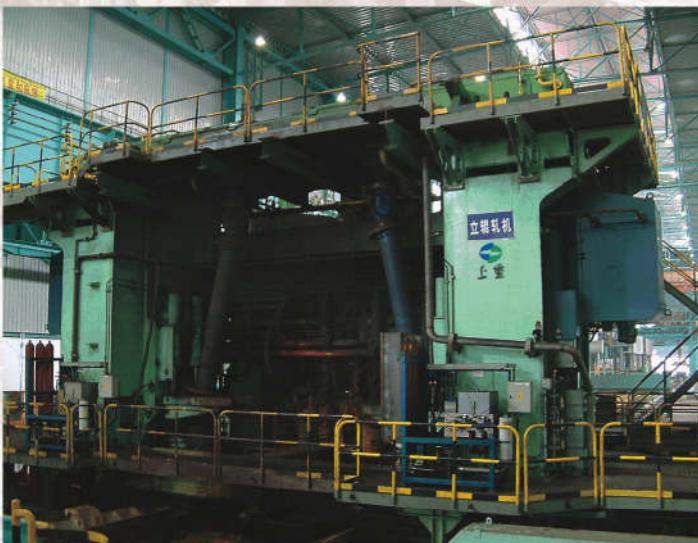
为沙钢制造的5000mm宽厚板立辊轧机 (一期) 5000mm heavy plate edger mill for Shagang Group (1st stage project)
