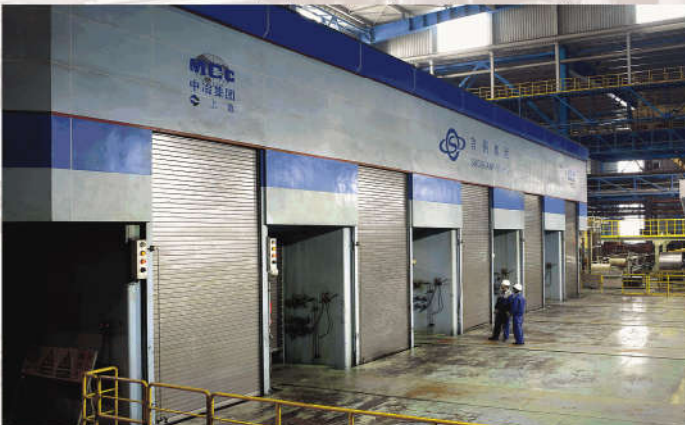
为首钢顺义制造的1850mm酸洗-冷连轧机组 (轧机段) 1850mm PL-TCM of rolling mill section for Shunyi, Shougang
