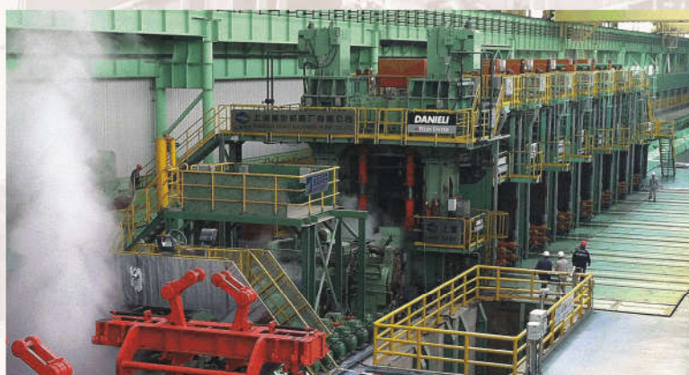
为宝钢梅钢制造的1780mm热连轧机组 (精轧区) 1780mm hot tandem rolling line (finishing mill section) for Meigang Baosteel
