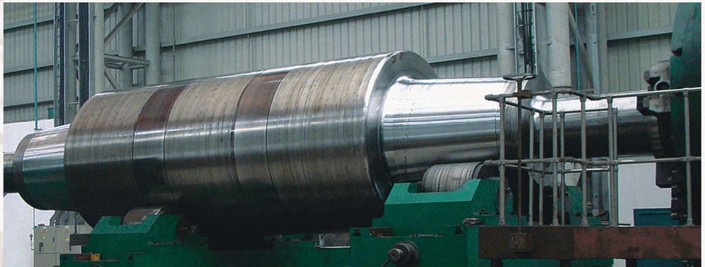
为首秦制造的4300mm宽厚板轧机支承辊 Back-up Roll of 4300mm 4-high Reversible Heavy plate Mill Shouqin Shougang
