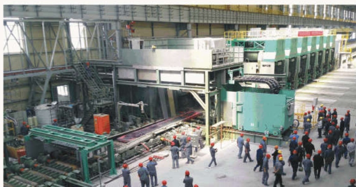
为山钢日照制造的2050mm热连轧机组 (精轧区) 2050mm hot tandem rolling line finishing mill section for Rizhao Sc steel
