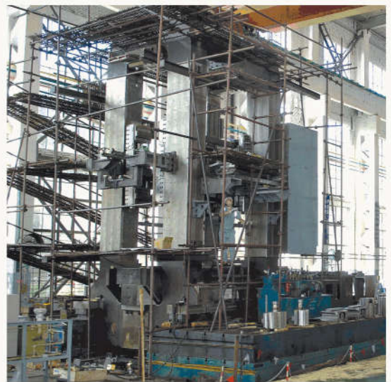
与日本SPCO公司联合设计并制造的台湾烨辉1700mm六辊可逆冷轧机组在上重工厂出厂装配 1700mm 6-high reversing cold rolling mill joint- designed with SPCO and manufactured for Yehui Taiwan assembly in SHMP for delivery
