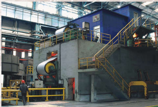
为包钢制造的1780mm酸洗—轧机联合机组 (酸洗段) 1780mm PL-TCM (pickling line equipments) for Bt Steel
