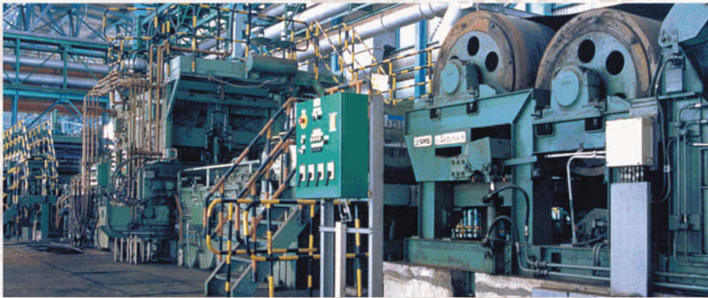
为宝钢制造的2030mm酸洗机组 2030mm continuous pickling line for Baosteel
