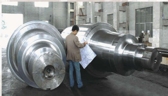
为西部材料制造的2800mm中厚板轧机支承辊 Back-up Roll of 2800mm 4-high Reversible Mill WMM Shaanxi
