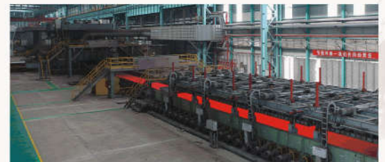
为莱钢制造的4300mm宽厚板ACC快速冷却设备 ACC equipments of 4300mm heavy plate mill for laiwu Steel
