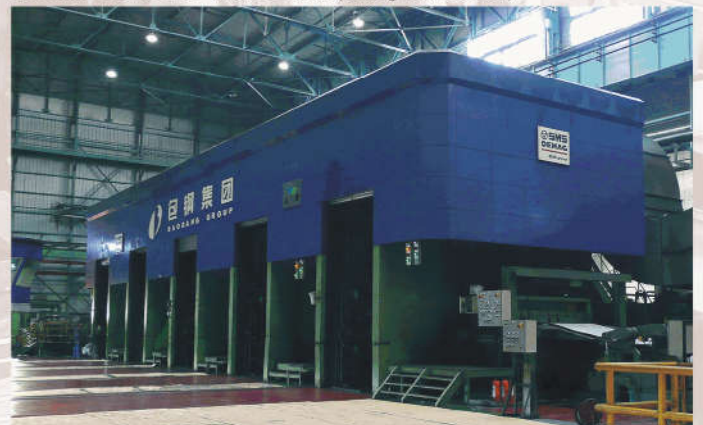
为包钢制造的1780mm酸洗-冷连轧机组 (轧机段) 1780mm PL-TCM of rolling mill section for Bt Steel
