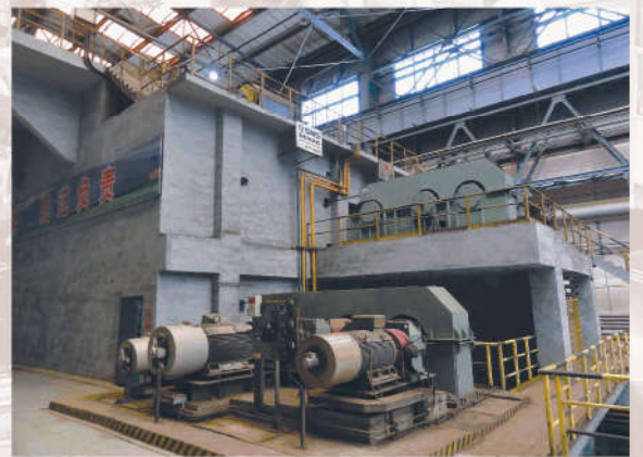
为包钢制造的1780mm酸洗—轧机联合机组 (酸洗段) 1780mm PL-TCM (pickling line equipments) for Bt Steel
