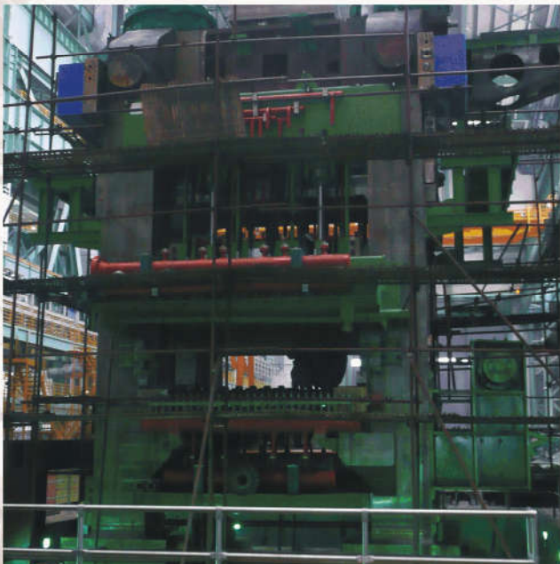
为济钢自主设计制造的3500mm中厚板粗轧机 在上重公司进行出厂装配 3500mm self-designed heavy plate roughing mill for Jigang, assembly in SHMP for delivery
