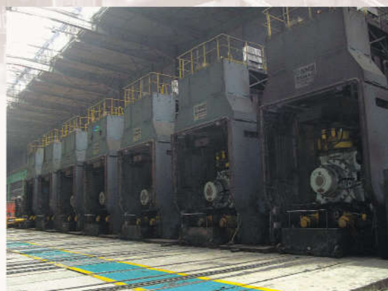
为首钢京唐制造的2250mm热连轧机组(精轧区) 2250mm hot tandem rolling line (finishing mill section) for Jingtang, Shougang
