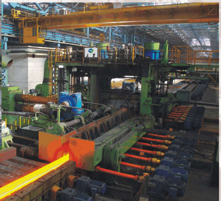
为包钢制造的百米重轨轨梁万能轧机 100m heavy rail beam universal mill-hot saw for Baotousteel
