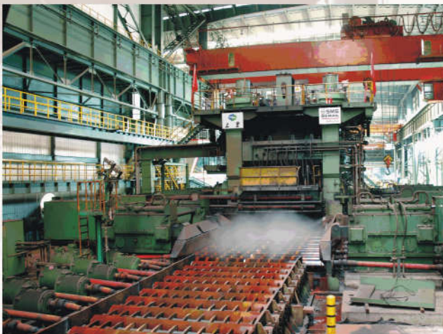
为包钢制造的3800mm宽厚板粗轧机 3800mm heavy plate roughing mill for Baotousteel
